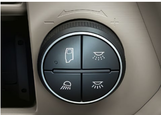
The rotary switch controls the light selection and dimming.
