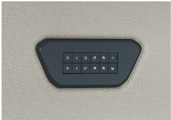
Central bed module provides easy access to vehicle functions including lighting, heating, radio and doors. Features can also be controlled using the MYIVECO Easy Way App.
