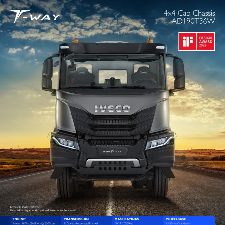
Power: 360hp (265kW) @ 2200rpm Torque: 1650Nm @ 925rpm
